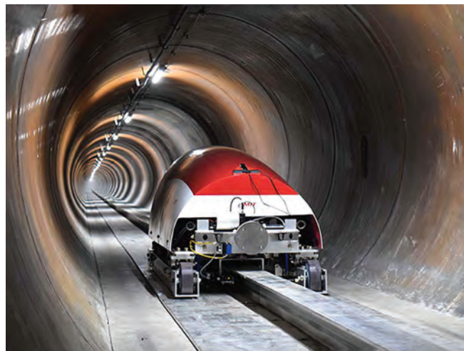
Magnetically-propelled transit pods for the Hyperloop on the California test track
